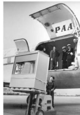
The IBM Model 350 disk file with a storage space of 5MB from 1956 and a Micro SD Card
